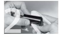
For maximum clamping forces, the bore, the tool shank, the cone of the clamping sleeve and the inner cone chuck must be degreased each time the tool is changed.
